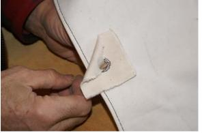
Now you are going to pull the square through to the other side of the tarp. Start by grabbing on a corner and pulling it through to the underside.
