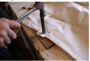
Cut or punch your grommet hole through the "square" and the tarp, being careful not to cut sewn threads.
